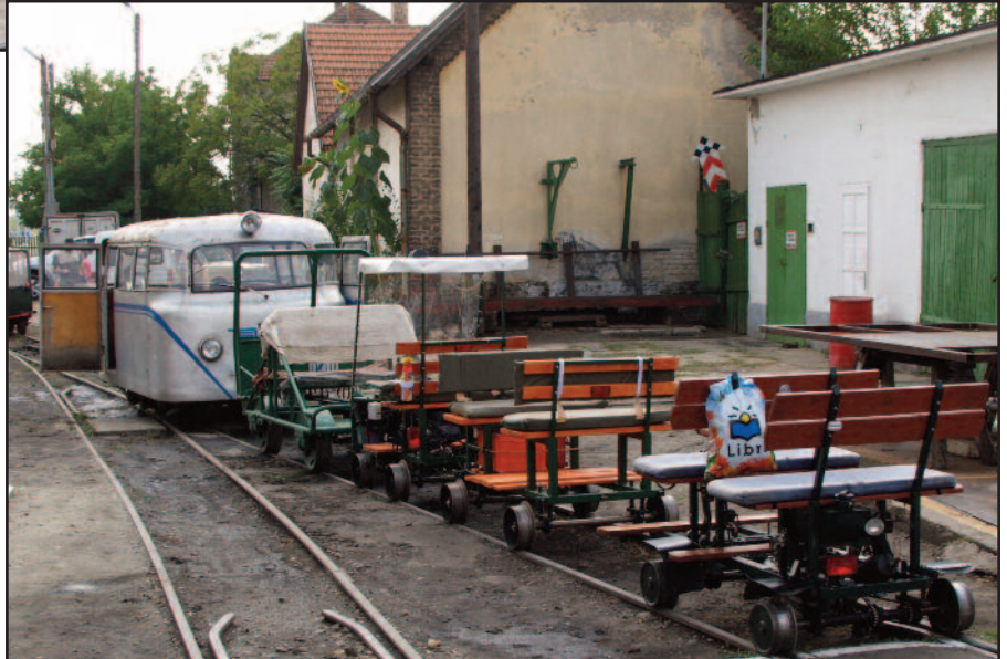
Above: The two oldest railcars in Hungary - the open car was “narrowed” down from a standard gauge PVG inspector’s railcar - the covered car is all original. Right: Home-built speeders at Kecskemét Narrow Gauge Railway, 55 miles southeast of Budapest. The silver car is Czech made.
