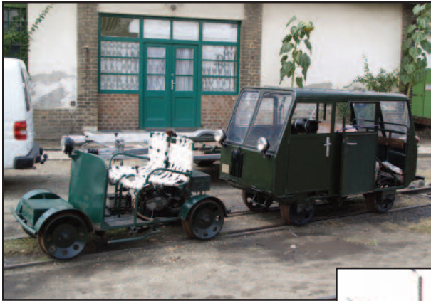
Above: The two oldest railcars in Hungary - the open car was “narrowed” down from a standard gauge PVG inspector’s railcar - the covered car is all original. Right: Home-built speeders at Kecskemét Narrow Gauge Railway, 55 miles southeast of Budapest. The silver car is Czech made.
